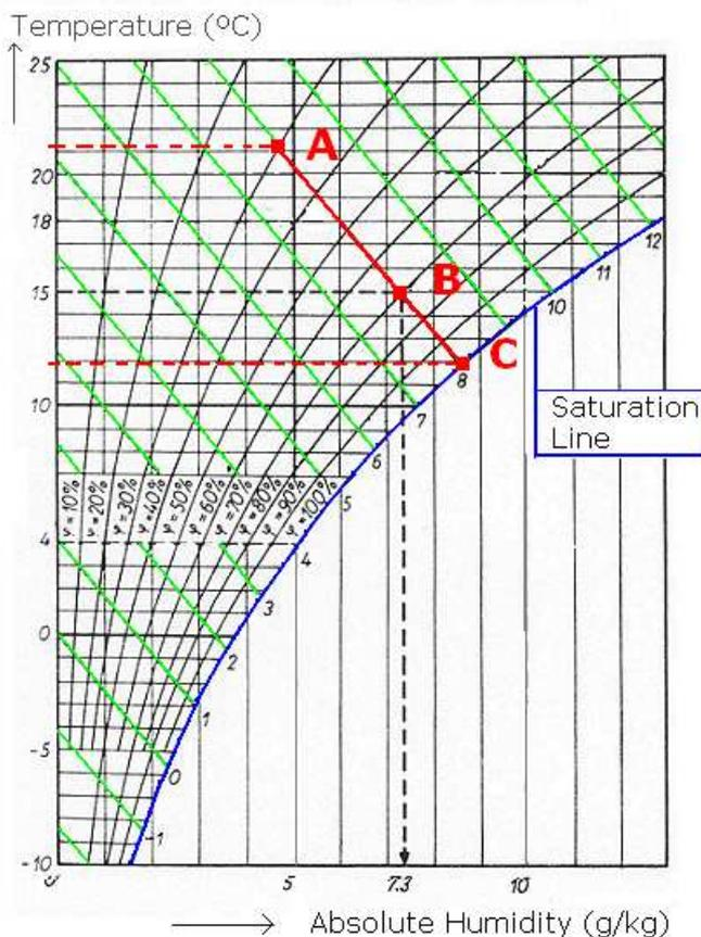
When water evaporates into this air, the condition of the air moves along a line of constant enthalpy (green lines). For perfect evaporative cooling the final condition is the dew point, which is the intersection of the enthalpy line and the saturation line (point "C"). The dew point in this case has a temperature of 11,7 °C and a water content
