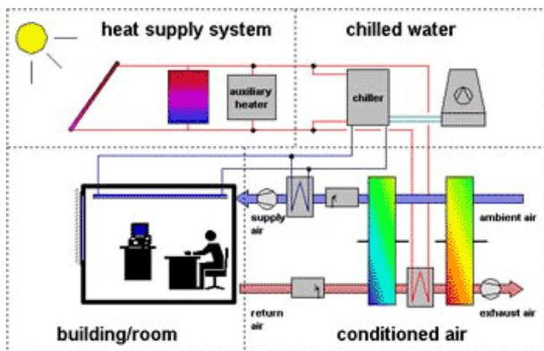
Figure 1. Solar thermal cooling system (figure: [www.californiasolarcenter.org](http://www.californiasolarcenter.org))
